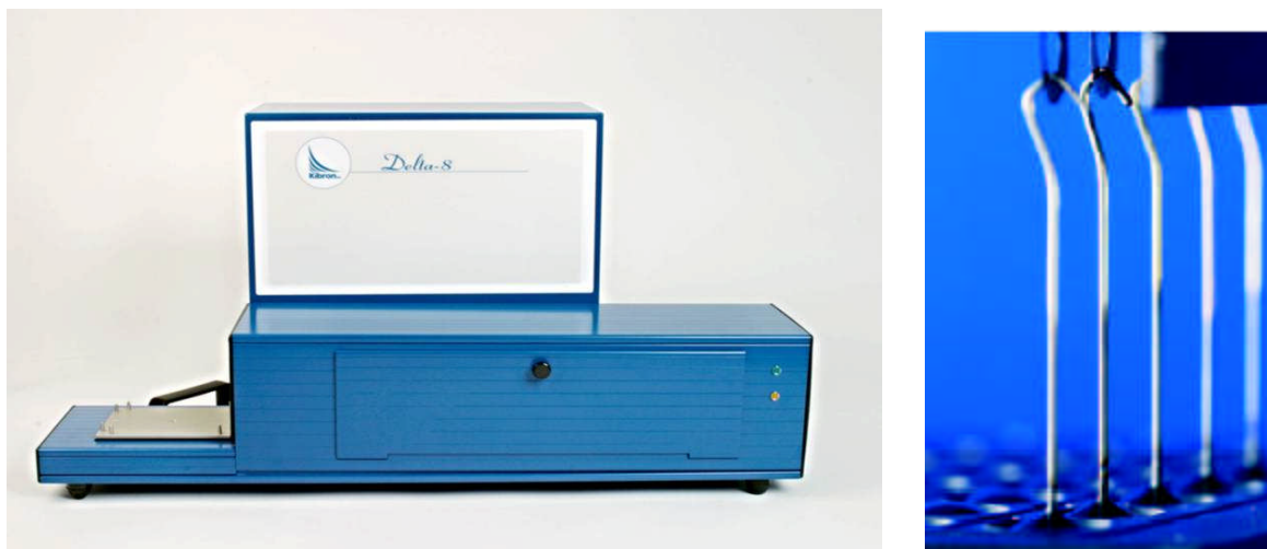
Figure 3. The Kibron Delta-8 multichannel tensiometer (left) and close-up view of the eight measurement probes (right). A 96-well plate is loaded on the left-hand side of the unit, and is automatically moved under the probes during a measurement.
